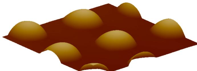
AFM picture of 140 micron microlens array. The non-symmetry is caused by the measurement error of AFM, which is ideal to measure the height differences but may have error during the measurement of continuous profiles
