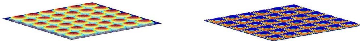
Illustration of refractive and diffractive microlens array
