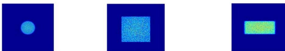
Output laser beam spots by diffusers
